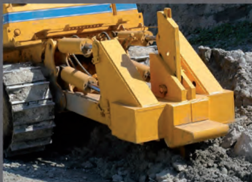
Single-shank and multi-shank rippers are equipped with hydraulic pitch.
